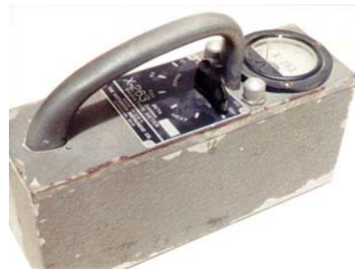
Figure 5: 1946 Victoreen model X-263 Geiger counter (ORAU)
