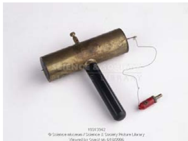
Figure 4: 1932 counter made by Hans Geiger (Science and Society Picture Library)
